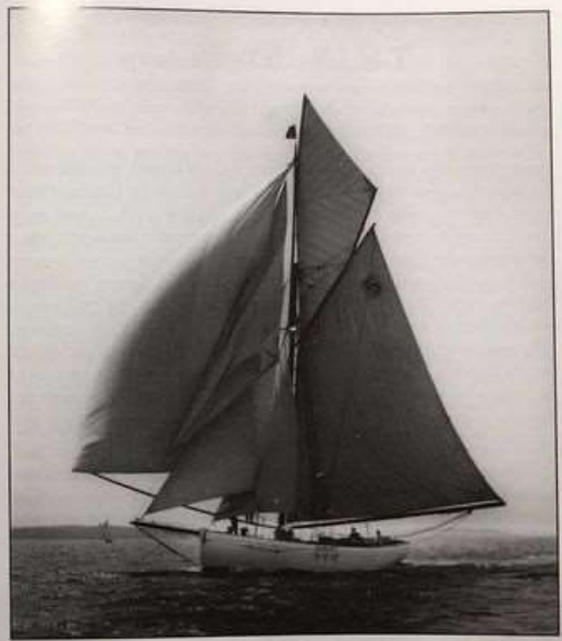
TALLY HO in 1927, running with spinnaker, showing off her en- larged rig with new mast and the addition of a spinnaker
